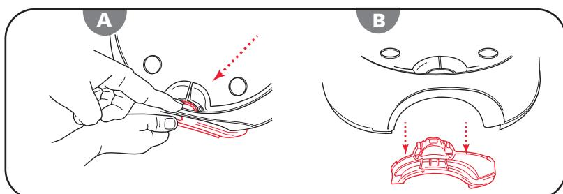
Disassembling the side joints for thorough cleaning.
