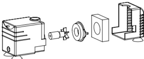
For best results, clean impeller and impeller well, every three (3) to six (6) months
